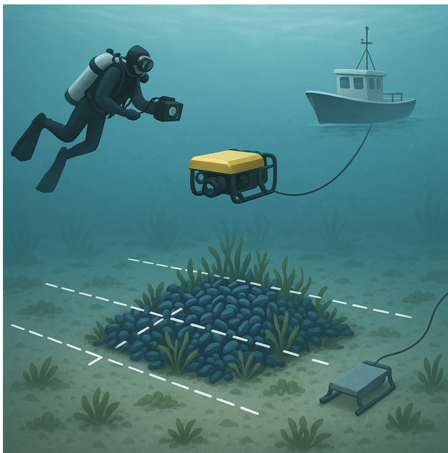
Figure 6. Schematic view of underwater video transects monitoring methods for blue mussel reefs. AI-generated image by OpenAI 2025.
