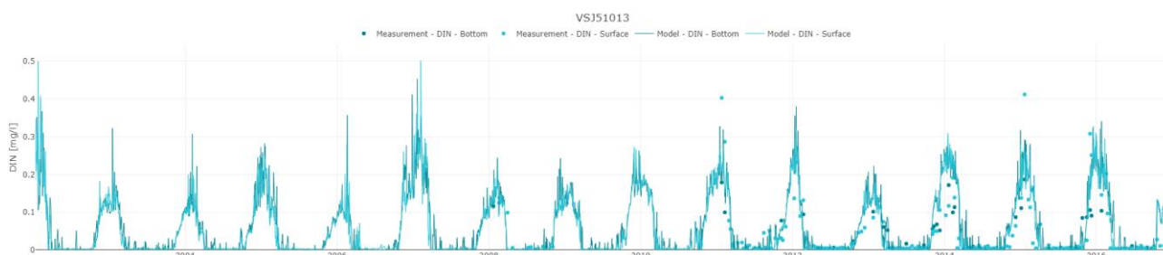
Figure 5-9 Measured and modelled concentrations of dissolved inorganic nitrogen (DIN, mg/l) at station VSJ51013 in the surface and bottom (2 m) waters. Dots represent measurements, and solid lines show modelled data for the entire period.
