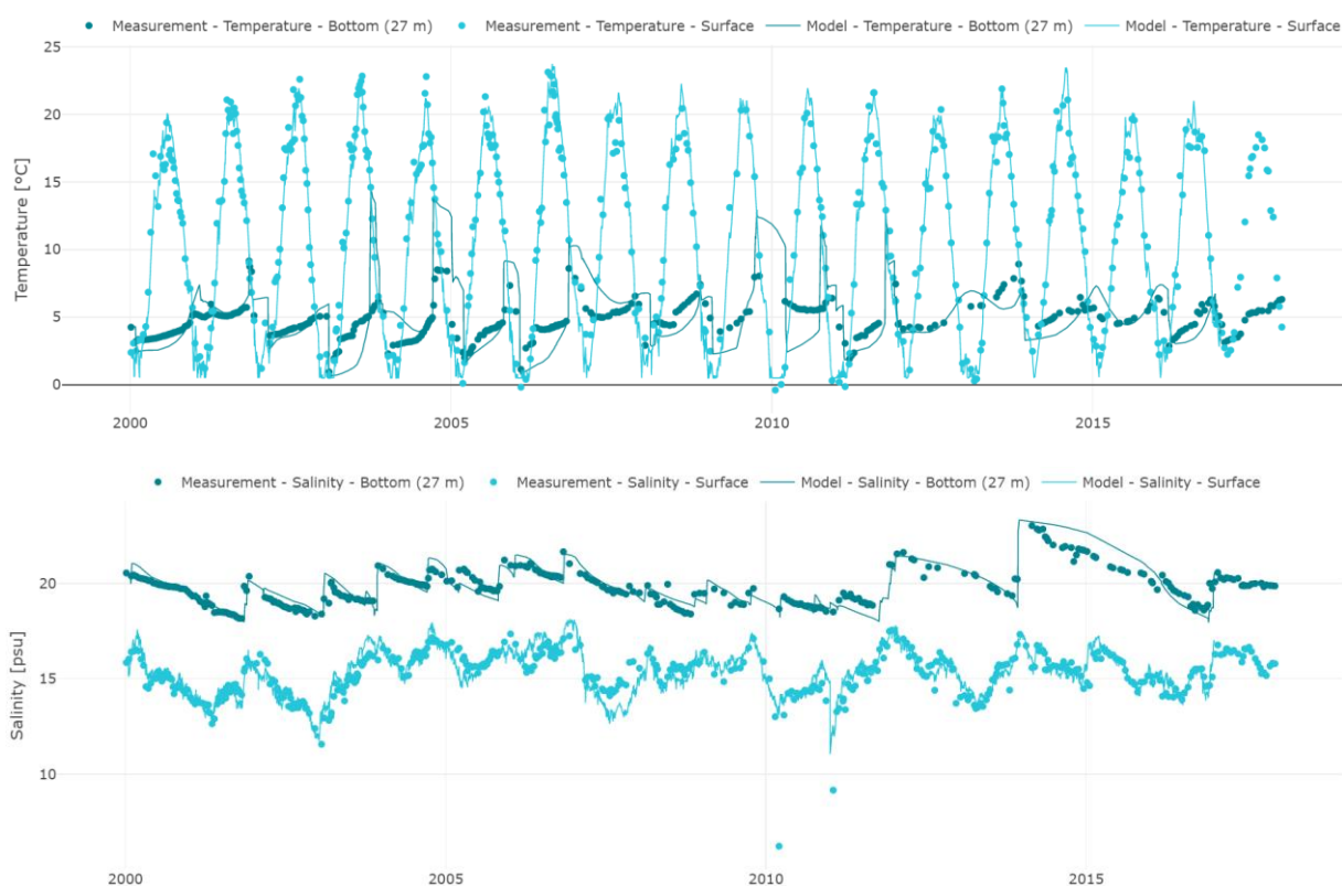
Figure 6-2 Comparison of measured and calculated water temperature (top panel) and salinity (bottom panel) at station NOR5503 for the model period 2002-2016. Data are also displayed at rbmp2021-2027.dhigroup.com .
