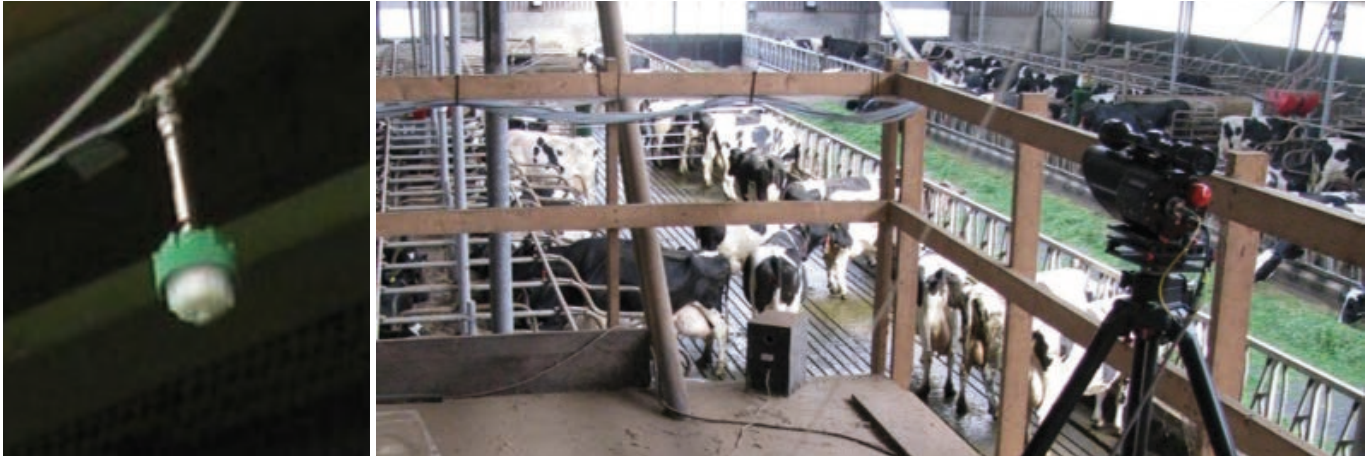
Figure 15: left: Sampling point with critical orifice and dust filter. Right: Open-path laser system.
