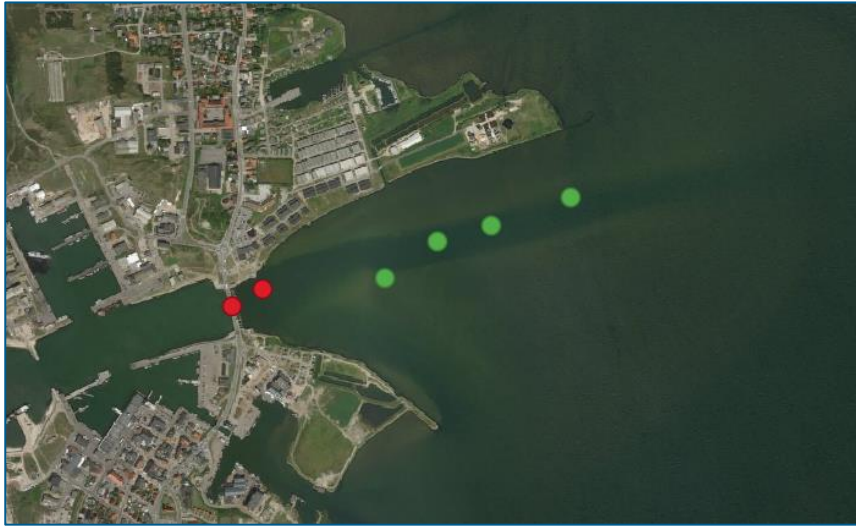
Figure 4.7 Location of sluice sources in Hvide Sande. Each red point represents five outflow sources, which were placed in sigma-layers 9-13. Each green point represents two or three inflow sources, which were placed in the sigma-layers 1-3.
