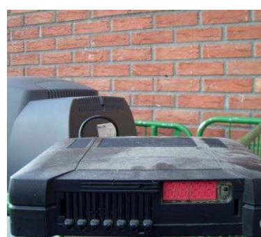
The display cover is missing
