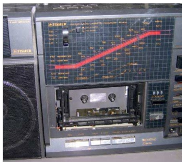
The cassette holder is missing
