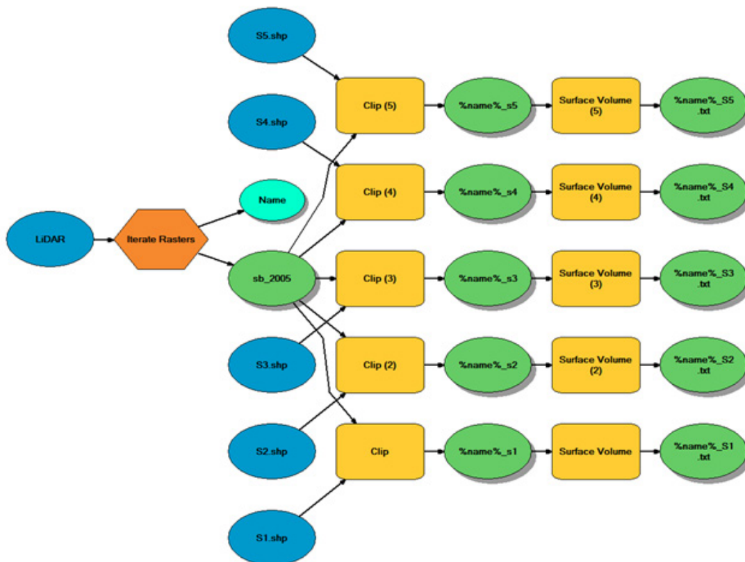
Figure 5-3. Model Builder created in ArcMap showing the work flow for volume analysis of the LiDAR scans using the surface volume tool.
