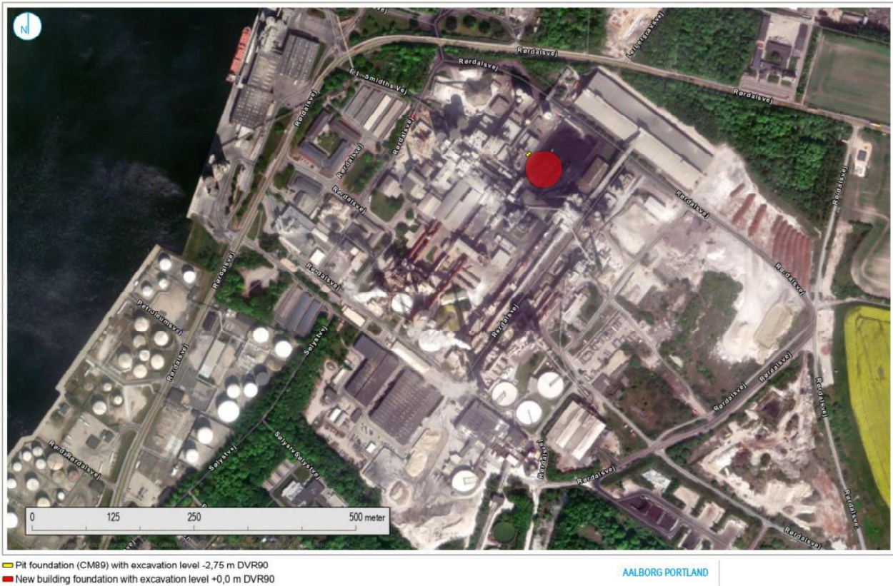
Figure 1-1 Overview of project location and two designated sites for excavation: one for the new building foundation and another for the pit foundation.
