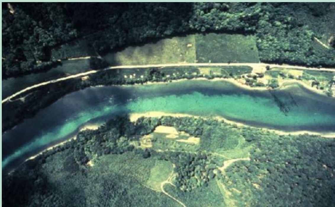
FIGURE 2. Illustration of contaminant mixing in the Rhine River by dye tracer experiment. Tracer is released from the left outside the picture (bright color), stream flows towards right. (Unknown source)
