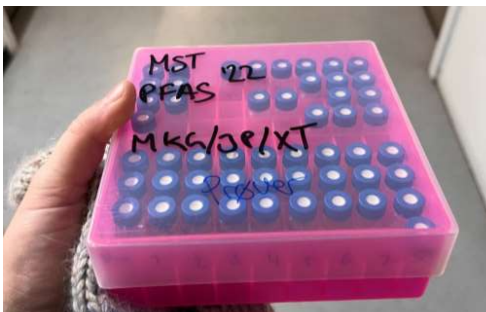
Figure A2: Precious final samples. Note that PFAS stick to surfaces, especially to glass and metal. To avoid losses, minimize the total surface area that PFAS are in contact with from sampling, sample pretreatment to analyses. To achieve the highest recovery, clean tubes with extra solvent and recombine with extract.
