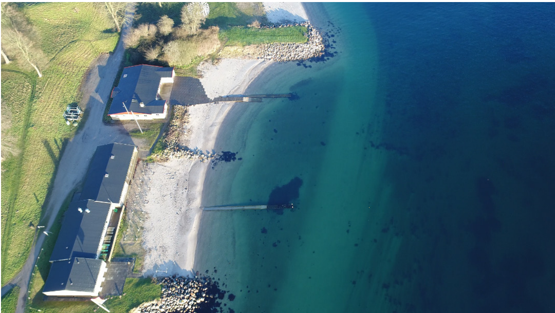
Figure 5.6: Frame extracted from the drone film made on the 02-01-2018. The image shows the rowing and kayaking club in the N-end of section 4. The longshore transport is evident in the sediment fan from the terminal groyne of section 3 towards S in section 4.
