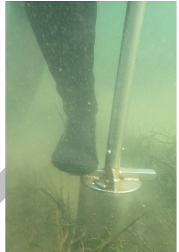
Figure 12. Example of a vacuum-based hand-held sediment corer.
