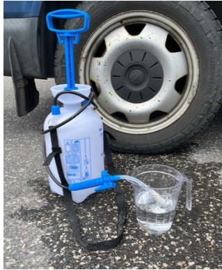
Figure 6. Water pump with silicone tubing and sterivex attached.
