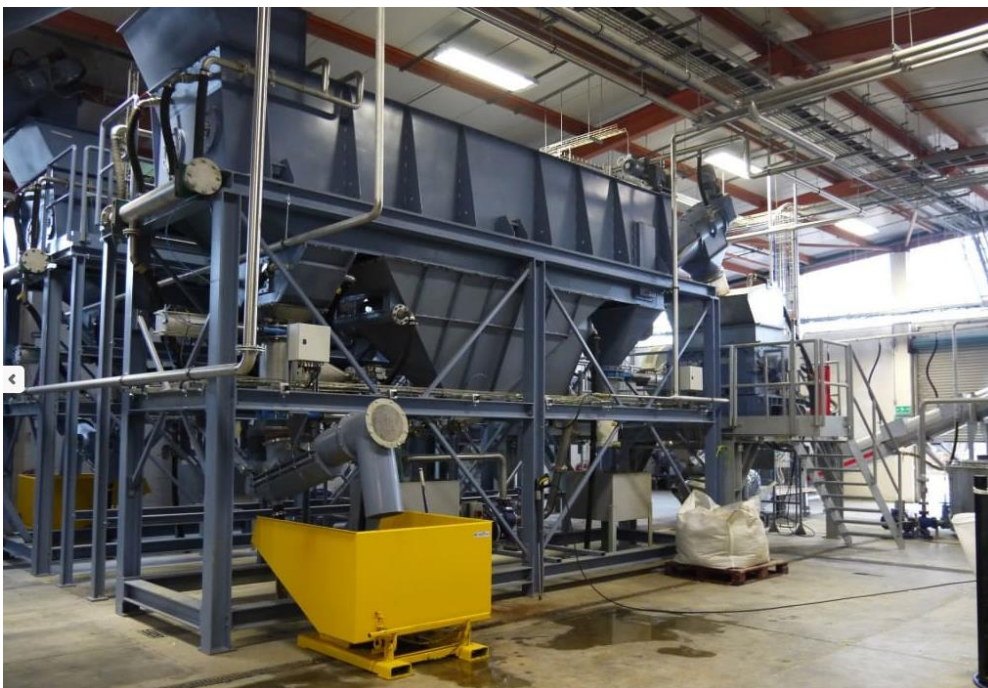
FIGURE 35: PHOTO PRE-WASH (SWIM-SINK) / COMPANY HERBOLD MECKESHEIM / PICTURE SOURCE: INTERNET
