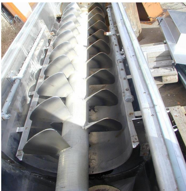
FIGURE 40: PHOTO FRICTION WASHER / COMPANY HERBOLD MECKESHEIM / PICTURE SOURCE: INTERNET
