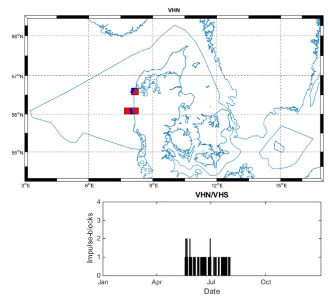
Subbottom profiling with magnitude **very low**. Conducted between 19.5.2017 and 2.8.2017. Source level given as 187 dB re. 1  $\mu$ Pa<sup>2</sup>s, 221 dB re. 1  $\mu$ Pa peak. 55 impulse-block days, distributed across three ICES subrectangles.
