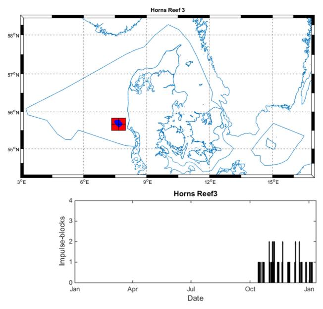
Pile driving of magnitude low (2500 kJ hammer energy), mitigated by means of a bubble curtain (Big Bubble Curtain). Conducted in period from 14.10.2017 to 5.1.2018. In total 49 impulse-block days in 2017, 4 impulse-block days in 2018, distributed over four ICES subrectangles.
