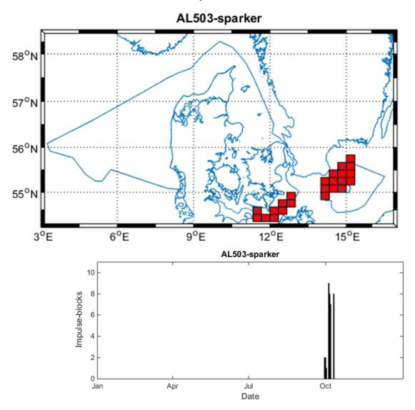
Subbottom profiling with sparker 8Innomar SES-2000 medium) of magnitude high. Conducted between 30.9.2017 and 11.10.2017 with a total of 37 impulse-block days.
